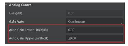
Figure 11-22 Set Gain under Once or Continuous Mode
